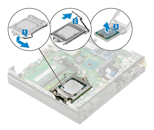
NOTE: After removing the processor, place it in an antistatic container for reuse, return, or temporary storage. Do not touch the bottom of the processor to avoid damage to the processor contacts. Touch only the side edges of the processor.
