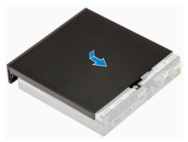
c Replace the thumbscrew to secure the cover to the system.
