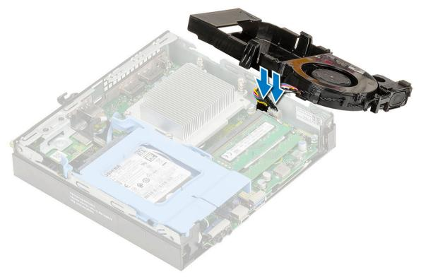
b Place the heat sink blower on the system and slide until it clicks into place.
