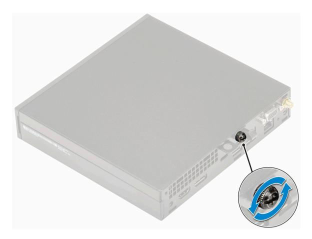
b Slide the side cover towards the front of the system and lift the cover to remove from the system.
