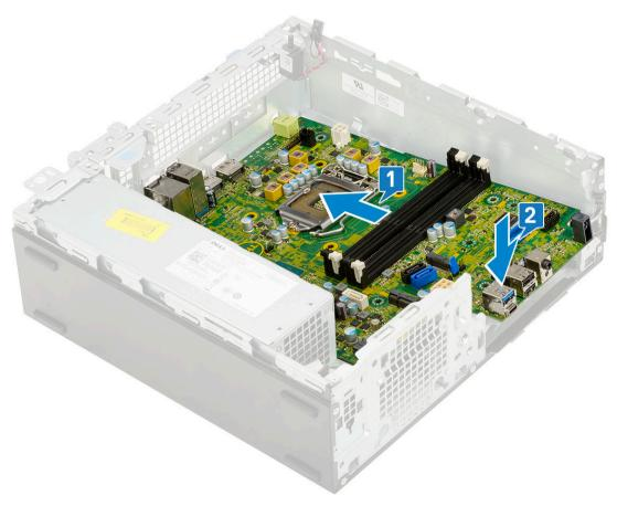
Replace the single (#6-32) screw, single (M3x5) screw and 5 screws that secure the system board to the system [1,2]. 3
