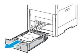
4. Remove any crumpled paper from the tray and any remaining paper jammed in the printer.
