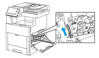
10. To reinsert the waste cartridge, lower the bottom of the cartridge into position. To lock the cartridge into place, push the top forward until the latch clicks into place.
