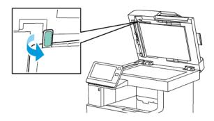
8. Using a soft cloth moistened with water, wipe the mirrored glass, the white-plastic strip, and the rollers. If dirt is difficult to remove, moisten a soft cloth with a small amount of neutral detergent, then wipe the printer parts dry with a soft cloth.
