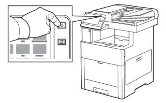
6. Configure the Wi-Fi settings from the front panel or the embedded web server if connected via ethernet. For more information, refer to Resetting Wireless Settings.
