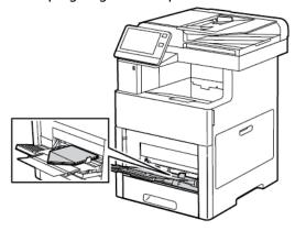
Load envelopes with the print-side up, flaps closed and down, and flaps going into the printer.
