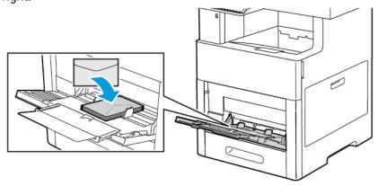
Load envelopes with the print-side up, flaps open and down, and the bottom of the envelope going into the printer.
