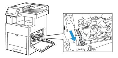
7. Insert the cleaning rod into one of the four cleaning holes until it stops, then pull out the rod. Repeat this two more times.
