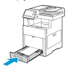
8. If the tray is extended for Legal-size paper, the tray protrudes when it is inserted fully into the printer. You can place a cover over the area protruding out of the tray.
