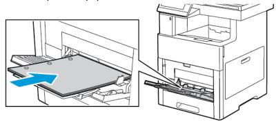
• For 1-sided printing, load letterhead or pre-printed paper face up with the top edge going into the printer.
