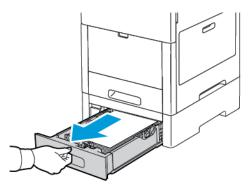
2. To remove the tray, lift the front of it slightly, then pull it out of the printer.
