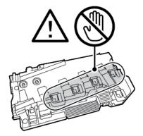
5. Place the removed waste cartridge on a level surface, with the openings facing up.
