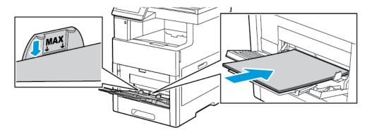
• Load hole-punched paper with the holes to the left.
