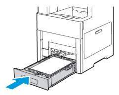
6. Insert the Bypass Tray completely into the printer.
