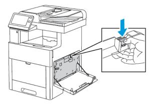
4. To remove the waste cartridge, lower the top of the cartridge and lift it away from the printer. To prevent toner spills, keep the openings facing up.
