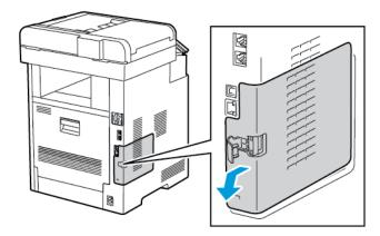
4. Reach into the printer and push the release lever toward the front of the printer. Hold the release lever in this position and gently pull the Wireless Network Adapter away from the printer.
