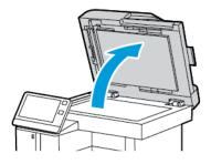
3. To access the jammed paper, open the Second-Side Scanning Access Cover, then remove any jammed paper.
