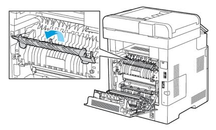
3. Remove any jammed paper from the back of the printer.
