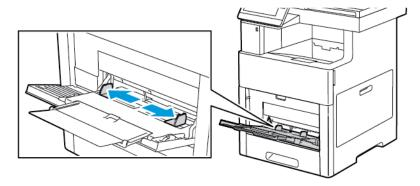
4. Load sheet-labels in the Bypass Tray, face up, with the top edge of the page feeding into the printer first.
