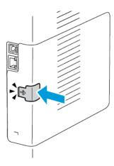
8. Connect the printer to your computer with a USB cable or to a network using an Ethernet cable.
