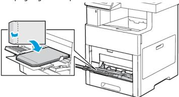
Load envelopes with the print-side up, flaps closed and down, and short edge going into the printer.
