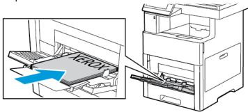
• For 2-sided printing, load letterhead and pre-printed paper face down with the top edge going into the printer.
