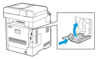
6. Place the left-side cover into place, then slide it toward the front of the printer.
