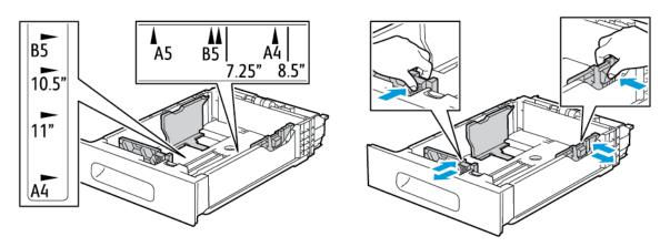
3. For Legal-size paper, to extend the front of the tray, press the green release latch, then pull the tray out.
