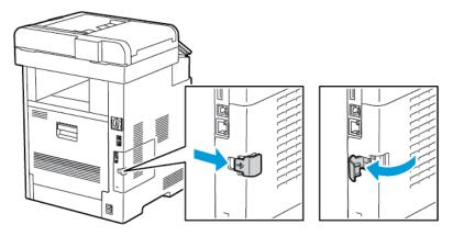
3. To remove the cover, slide it toward the back, then away from the printer.
